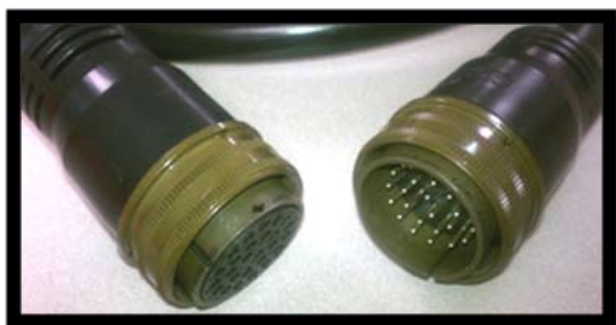
Figure 7. Cable with aluminum cable coupler ring.
